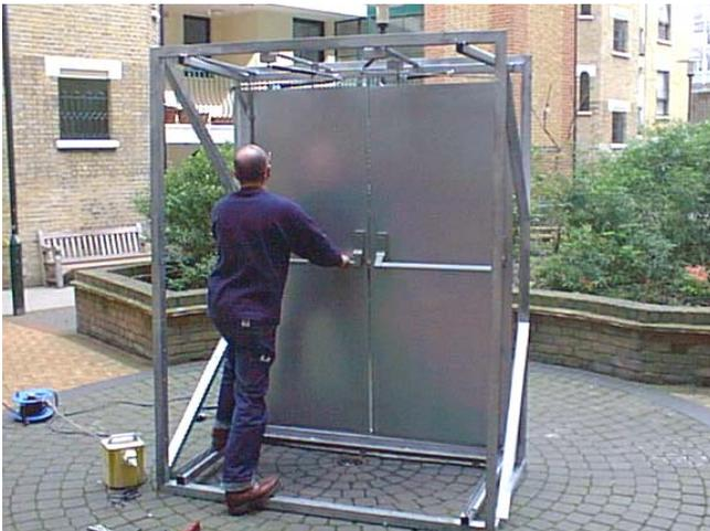
Generally, building out the recess will achieve the objective. However, in many licensed premises etc with more than 60 people exiting a building, fire exits require recesses under Fire Regulations. Under the Lilac Project and now being developed with the BRE/Global Construction and Camden/Westminster Police we are developing innovative fire exit doors for this type of building
